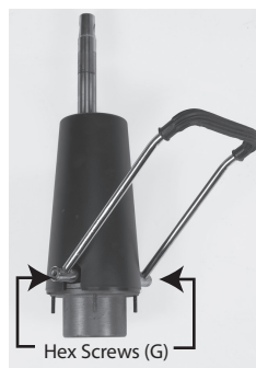
2. Attach the Pump Lever (L) to the Pump Base (I). Use the two Hex Screws (G) and the Allen Wrench (F) to secure Pump Lever (L) to Pump Base (I). The Hex Screws (G) should be slotted into the holes on the outer ends of the Pump Lever (L).
